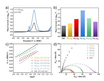
**Fig. 2** (a) CVs of  $Pd_1Ag_1$  NPs and commercial Pd/C in 1 M KOH and 1 M EG solution at 10 mVs<sup>-1</sup>; (b) comparison of peak mass currents of  $Pd_xAg_y$  NPs and commercial Pd/C; (c) Tafel slope plots and (d) Nyquist plots of  $Pd_xAg_y$  NP samples and commercial Pd/C in 1 M KOH containing 1 M EG.
