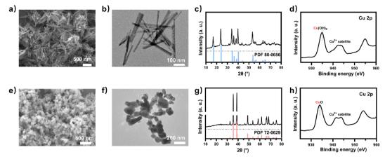
Fig. 3 (a) SEM image and (b) TEM image of Cu(OH)<sub>2</sub>. (c) XRD revealed peaks assignable to the pattern of Cu(OH)<sub>2</sub> (reference peaks from JCPDS Data Card No. 80-0656 given as drop lines). (d) XPS spectra of Cu 2p for Cu(OH)2. (e) SEM image and (f) TEM image of the model electrocatalyst CuO. (g) XRD revealed peaks assignable to the pattern of CuO (reference peaks from JCPDS Data Card No. 72-0629 given as drop lines). (h) XPS spectra of Cu 2p for CuO.
