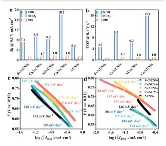
Fig. 5 Comparison of the  $J_k$  (a) and TOF (b) values of the catalysts at 0.1 V in 0.1 M KOH, HClO<sub>4</sub>, and PBS media. Tafel plots of the disk current density (c) and ring current density (d) at a rotating rate of 1600 rpm in the O2-saturated 0.1 M KOH media.
