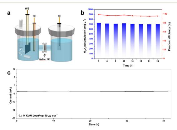
Fig. 8 (a) Schematic of the bulk H<sub>2</sub>O<sub>2</sub> production device. (b) The FE% and concentration of the produced H<sub>2</sub>O<sub>2</sub> using CA-NR. (c) Long-term stability test of CA-NR at 0.65 V.
