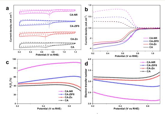
Fig. 6 (a) Cyclic voltammograms of samples in  $O_2$ -saturated 0.1 M KOH at 10 mV s<sup>-1</sup>. (b) Polarization curves of samples at 1600 rpm in  $O_2$ -saturated 0.1 M KOH (dashed lines: ring current; solid lines: disk current). (c)  $H_2O_2$  selectivity of samples. (d) Electron transfer number of samples.
