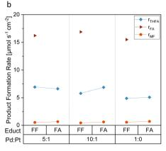
Fig. 6 Comparison of FF and FA as starting material with selected Pd: Pt on GC electrodes. (a) Reaction performance parameters and (b) product formation rates. With 0.05 M FF respectively FA solution in 0.5 M H<sub>2</sub>SO<sub>4</sub> electrolyte with 15% acetonitrile under galvanostatic conditions with –300 mA and 6 FEq transferred electrons.
