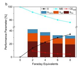
Fig. 2 (a) Concentration profile and (b) reaction performance parameters of the hydrogenation reaction of FF on platinized platinum (Pt/Pt) electrodes under variation of the total amount of transferred charge with 0.05 M FF solution in 0.5 M  $H_2SO_4$  electrolyte with 15% acetonitrile under galvanostatic conditions with -300 mA.
