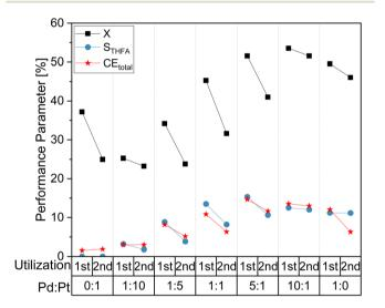
Fig. 4 Comparison of selected reaction performance parameters for the first and second utilization of different electrode material compositions. With 0.05 M FF solution in 0.5 M  $H_2SO_4$  electrolyte with 15% acetonitrile under galvanostatic conditions with -300 mA and 6 FEq transferred electrons.
