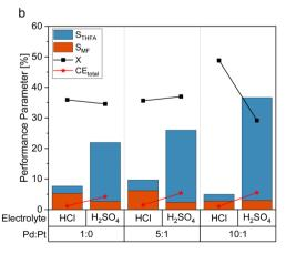
Fig. 5 Comparison of selected reaction performance parameters for the utilization of 0.5 M HCl solution and 0.5 M H<sub>2</sub>SO<sub>4</sub> solution with 15% acetonitrile for the utilization of (a) furfural and (b) furfuryl alcohol as starting material with 0.05 M FF solution under galvanostatic conditions with -300 mA and 6 FEq transferred electrons.
