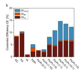
Fig. 3 Comparison of different working electrodes for their reaction performance indicators ((a) X and S, (b) CEs), including metal sheet electrodes (Pd, Pt), platinized platinum sheet (Pt/Pt), and Glassy Carbon (GC) electrodes coated with catalytic inks containing varying Pd: Pt ratios. With 0.05 M FF solution in 0.5 M H<sub>2</sub>SO<sub>4</sub> electrolyte with 15% acetonitrile under galvanostatic conditions with -300 mA, and 6 FEq transferred electrons.
