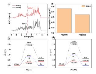
Fig. 5 (a) Projected density of states of Pb(111) and Pb(200). (b) The adsorption energies of \*OCHO on Pb(111) and Pb(200). Calculated Gibbs free energy diagrams of \*OCHO, \*COOH, and \*H on (c) Pb(111) and (d) Pb(200).
