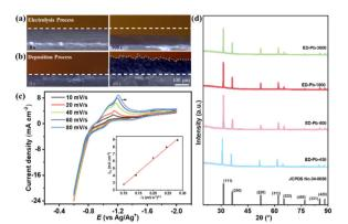
Fig. 1 In situ OM images of the Pb planar electrode in 0.5 M [Bmim][TFA]/AcN electrolyte (a) at -0.1 A for 900 s in the electrolysis process and (b) at 0.1 A for 900 s in the electrodeposition process. (c) Cyclic voltammograms of the Pb planar electrode at -0.6 to -2.0 V after the Pb electrolysis process (the inset illustration: relationship between  $\sqrt{v}$  and  $j_{\rm pc}$ ). (d) XRD patterns of the Pb standard PDF card (No. 04-0686) and ED-Pb electrodes with different deposition times.
