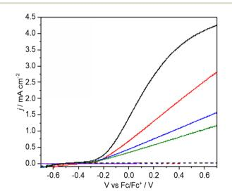
Fig. 2 Linear sweep voltammograms of  $BiVO_4$  photoelectrodes in electrolytes containing 2 M (black line), 1 M (red), 0.5 M (blue), 0.25 M (green), and 0.01 M (purple) PAA with 0.05 equiv.  $NEt_3$ . Voltammograms were recorded in the dark (dashed) and under 450 nm LED illumination (solid). Scan rate 10 mV s<sup>-1</sup>.
