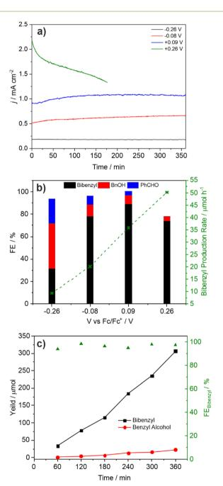
Fig. 3 (a) CPE of 1 M PAA with 0.05 equiv.  $Et_3N$  at -0.26 (black), -0.08 (red), +0.09 (blue) and +0.26 V (green) vs.  $Fc/Fc^+$ ; (b) faradaic efficiencies for bibenzyl (black), benzyl alcohol (red) and benzaldehyde (blue) as a function of electrolysis potential; (c) time-dependent bibenzyl (black) and benzyl alcohol (red) formation at +0.09 V vs.  $Fc/Fc^+$  of 1 M PAA with 0.05 equiv.  $Et_3N$ . Overall faradaic efficiency for bibenzyl is given in green.
