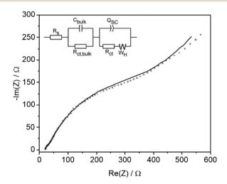
**Fig. 6** Nyquist plot and equivalent circuit for of an illuminated (450 nm,  $32 \text{ mW cm}^{-2}$ ) BiVO<sub>4</sub> photoanode in 0.05 M 4-Cl PAA solution with 0.05 equiv. Et<sub>3</sub>N containing 0.1 M TBAPF<sub>6</sub> supporting electrolyte at -0.06 V vs. Fc/Fc<sup>+</sup>. Data were acquired between 500 kHz-50 mHz, using an a.c. potential amplitude of 10 mV. Simulated impedance spectra are shown by the solid lines.
