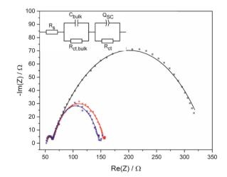
Fig. 4 Nyquist plot and equivalent circuit for of an illuminated (450 nm,  $32 \text{ mW cm}^{-2}$ ) BiVO<sub>4</sub> photoanode in 1 M 4-Cl PAA with 0.05 equiv. Et<sub>3</sub>N at -0.26 (grey circles), -0.06 (red) and 0.14 V (blue). Data were acquired between 500 kHz-50 mHz, using an a.c. potential amplitude of 10 mV. Simulated impedance spectra are shown by the solid lines.
