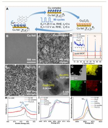
Fig. 1 (A) Schematic diagram of the preparation of the  $Cu_xC_yO_z$  catalyst. SEM images of (B) Cu foil, (C) Cu complex, and (E)  $Cu_xC_vO_z$ . (D) XRD patterns of different samples. (F) HR-TEM image and (G) elemental mappings images of Cu<sub>x</sub>C<sub>y</sub>O<sub>z</sub>. (H) The quasi in situ XPS signals of Cu Auger LMM spectra for the Cu foil, Cu complex, and  $Cu_xC_yO_z$ . (I) XANES spectra and (J) XES spectra of different samples.
