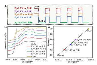
Fig. 2 (A) Schematic diagram of the preparation of the  $Cu_xC_yO_z$  catalyst under different conditions ( $E_a=1.0\ V$ , 1.25 V, 1.4 V, and 1.6 V vs. RHE,  $t_a=3\ s$ ,  $E_c=-1.0\ V$  vs. RHE,  $t_c=5\ s$ ). (B) XANES spectra at the Cu K-edge under different conditions. (C) Average oxidation state of Cu in  $Cu_xC_yO_z$  under different conditions from Cu K-edge XANES.
