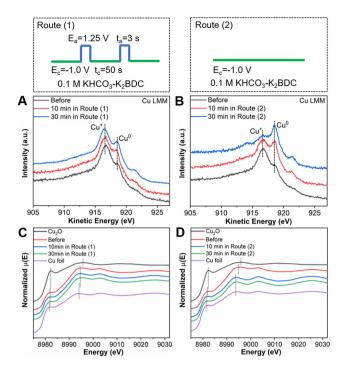
Fig. 3 The quasi *in situ* Auger LMM spectra of Cu for  $Cu_xC_yO_z(0.41)$  reacted in (A) route (1) and (B) route (2) for different times. The *in situ* XANES spectra of  $Cu_xC_yO_z(0.41)$  reacted in (C) route (1) and (D) route (2) for different times.
