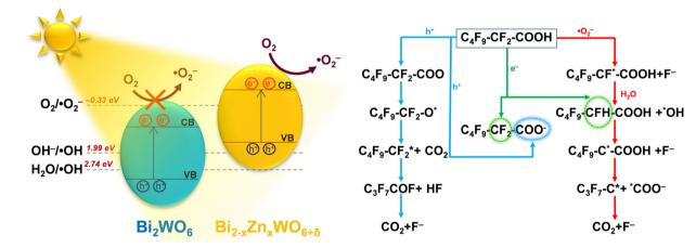
Fig. 8 Possible mechanism for the photodegradation of PFH<sub>x</sub>A in an aqueous solution over the Zn<sup>2+</sup>-substituted Bi<sub>2</sub>WO<sub>6</sub> photocatalyst.
