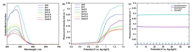
Fig. 5 (a) UV-vis diffuse reflectance spectra of  $Bi_{2-x}Zn_xWO_{6+\delta}$  powders with varying contents of  $Zn^{2+}$  substituent. Photoelectrochemical results of  $Bi_{2-x}Zn_xWO_{6+\delta}$  as photoanodes in 0.1 M  $Na_2SO_4$  deoxygenated water solution: LSV (b) and CA (c) at 1.4 V (V vs. Ag-AgCl) for Zn0 and Zn2.5.
