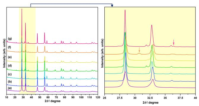
Fig. 1 XRD patterns of  $Bi_{2-x}Zn_xWO_{6+\delta}$  powders with varying contents of  $Zn^{2+}$  substituent: (a) Zn0, (b) Zn1, (c) Zn2.5, (d) Zn7.5, (e) Zn12.5, (f) Zn17.5, and (g) Zn22.5. The orange and magenta arrows indicate the reflections belonging to ZnWO₄ and ZnO, respectively.
