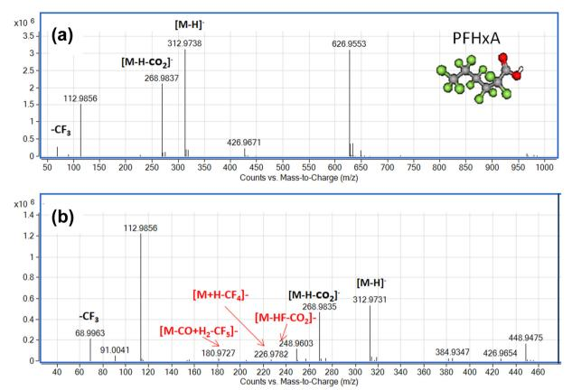
Fig. 7 Mass spectra of PFH<sub>x</sub>A-containing water samples before (a) and after (b) photocatalytic treatment in the presence of sample Zn2.5.
