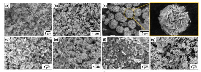
Fig. 3 SEM images of Bi<sub>2-x</sub>Zn<sub>x</sub>WO<sub>6+3</sub> powders with varying contents of Zn<sup>2+</sup> substituent: (a) Zn0, (b) Zn1, (c) Zn2.5, (d) Zn7.5, (e) Zn12.5, (f) Zn17.5, and (g) Zn22.5.
