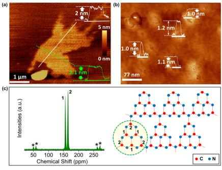
Fig. 2 (a) AFM image of g-CN nanosheet with sectional profile measurement showing height and thickness profiles (nm). (b) AFM images of nanosheets with respective height profiles at different locations. (c) Solid-state <sup>13</sup>C NMR spectra of as-prepared g-CN and its idealized structure showing heptazine tectonic units.
