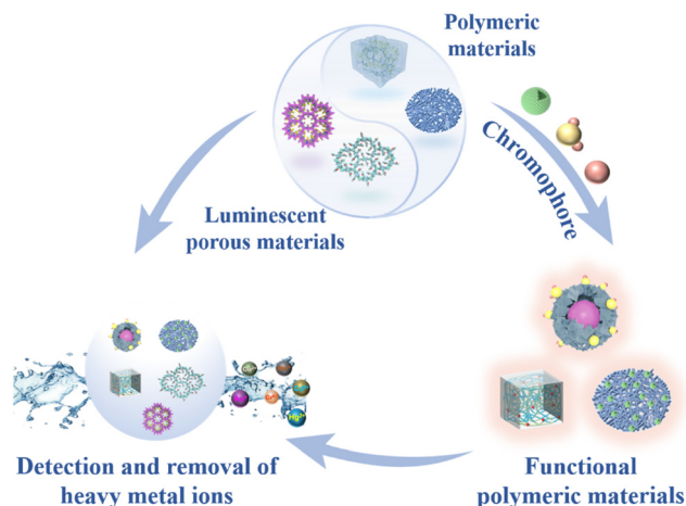
Fig. 1 Schematic diagram of functional materials fabrication and their applications for detection and removal of heavy metal ions.
