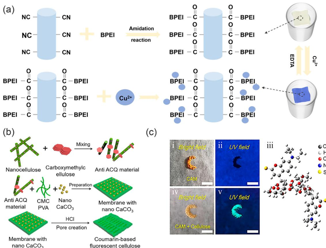
**Fig. 13** The sensing and removal mechanism of functional polymer membranes for heavy metal ions in. (a) The preparation of aPAN/BPEI NMs and detection/removal of  $\text{Cu}^{2+}$ . Reproduced from ref. 107 with permission from American Chemical Society. Copyright 2021. (b) The preparation of anti-ACQ materials. (c) The optical image of CAM under natural light and ultraviolet light and the optical image of anti-ACQ material under natural light and ultraviolet light.
