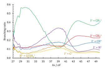
Fig. 4 Double ionization branching ratios plotted for the observed ion pairs as detected by PEPIPICO in the 27–50 eV photon energy range.
