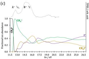
Fig. 1 (a) Overall iodomethane breakdown diagram in the 11–43 eV range with the sum of the minor fragment ions plotted together. (b) The minor channels plotted separately for better legibility together with the thermochemical thresholds to HI+ and H+ formation. (c) Fragment ion abundances summed into  $CH_n^+$ ,  $CH_nI^+$  and  $I^+$  groups (see text), shown together with the TPES in the 11.5-22.0 eV range
