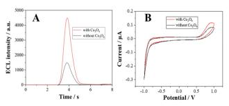
Fig. 1 (A) ECL profiles and (B) CV curves of the L012-H<sub>2</sub>O<sub>2</sub> system at the ITO surface with and without  $Co_3O_4$ . Working solution: 10 mM PBS containing 200  $\mu$ M L012. Scan range: -1.0 to 1.0 V, scan rate: 0.1 V s<sup>-1</sup>, PMT voltage: 600 V.
