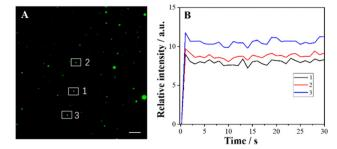
Fig. 4 (A) ECL image of  $Co_3O_4$  at ITO slides; (B) the fluctuation of ECL intensity at three particles labeled as 1, 2 and 3 in (A). The exposure time was 500 ms; the applied potential was 1 V. Scale bar: 5  $\mu$ m.
