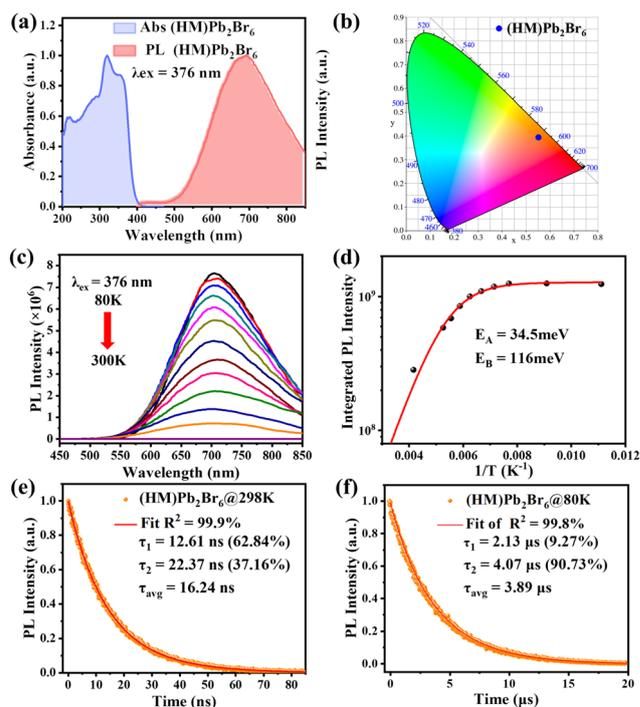
**Fig. 2** (a) Normalized absorption and PL spectra of (HM)Pb<sub>2</sub>Br<sub>6</sub>. (b) The CIE 1931 chromaticity coordinate. (c) Temperature-dependent PL spectra of (HM)Pb<sub>2</sub>Br<sub>6</sub>. (d) Integrated PL intensity as a function of reciprocal temperature. Time-resolved PL decay curve of (HM)Pb<sub>2</sub>Br<sub>6</sub> under a 375 nm excitation laser line at (e) 298 K and (f) 80 K.
