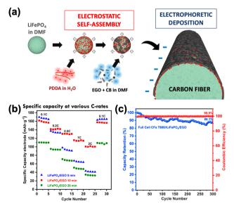
Fig. 10 (a) Schematic illustration of EPD synthesis of the LiFePO<sub>4</sub>/EGO electrode composite. (b) Specific capacities (normalized over the total mass of both electrodes, anode and cathode) at various C-rates. (c) Cycling performance and Coulombic efficiency at 1C. Reproduced with permission.<sup>6</sup> Copyright 2021, Elsevier.
