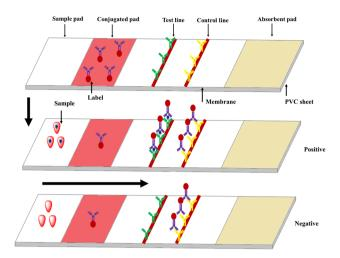
Fig. 4 Typical immunochromatographic assay format.
