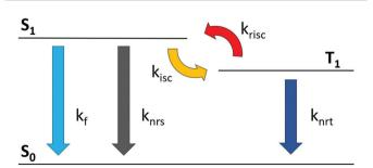
Fig. 1 Schematic illustration of the TADF model described in this study. So is the singlet ground state,  $S_1$  and  $T_1$  are the singlet and triplet excited states. Five processes are considered: radiative and non-radiative decay of  $S_1$  ( $k_f$ ;  $k_{nrs}$ ), intersystem-crossing ( $k_{isc}$ ), reverse intersystem-crossing ( $k_{risc}$ ) and non-radiative decay of  $T_1$  ( $k_{nrt}$ ).
