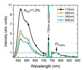
**Fig. 8** UC spectra of the optimized PS:**PdPc/Rub** films with different sensitizer layer thicknesses (indicated). The spectra are normalized to FL**PdPc** peak intensity (at 774 nm) so that UC intensity would correspond to  $\phi_{\rm UC}$ . Excitation wavelength and density, 730 nm and 100 W cm<sup>-2</sup>, respectively.
