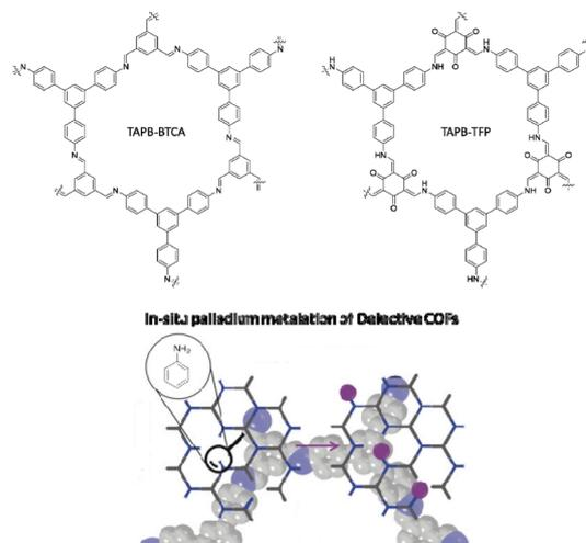
Fig. 38 Structure of TAPB-BTCA and TAPB-TFP COFs.
