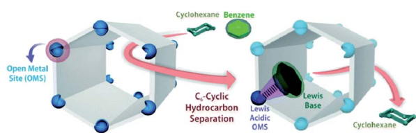
Fig. 2 Role of metal site in MOF-74 towards the separation of benzene from cyclohexane. Reproduced/adapted from ref. 56 with permission from The Royal Society of Chemistry. 56
