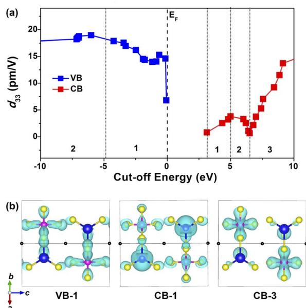
Fig. 7 Theoretical analysis of the SHG source for SrCdSi<sub>4</sub>: (a) variation of cut-off energy (eV) versus the largest static  $d_{33}$ ; (b) charge-density maps in the selections (VB-1, CB-1, CB-3) of major contribution. Black atoms: Sr; blue atoms: Cd; pink atoms: Si; yellow atoms: S.
