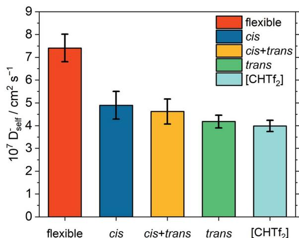
Fig. 14 Anion self-diffusion coefficients obtained from MD simulations of native, flexible  $[\text{C}_4\text{C}_1\text{im}][\text{NTf}_2]$ , compared with targeted modifications where the anions in the simulation are restrained to *cis*/*trans* conformers. The ionic liquid  $[\text{C}_4\text{C}_1\text{im}][\text{CHTf}_2]$  is shown for comparison.
