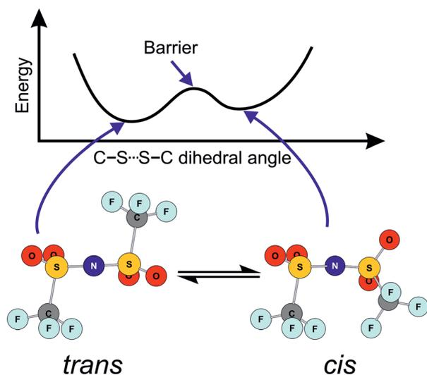
Fig. 1 Schematic of the two minimum energy conformers of the  $[\text{NTf}_2]^-$  anion, and of the energy as a function of the C–S...S–C dihedral angle. Adapted from ref. 39.
