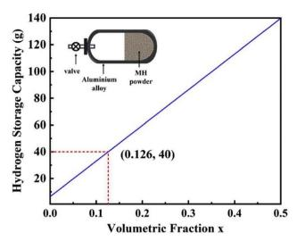
Fig. 6 Relationship between the hydrogen storage capacity and the volume of the filled alloys in a 4 MPa low-pressure hybrid tank.<sup>90</sup>
