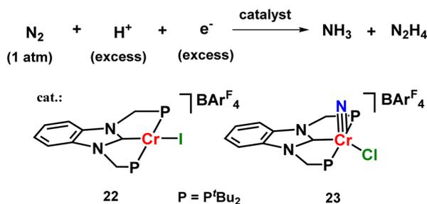
Fig. 28 Chromium complexes towards catalytic N<sub>2</sub> fixation.
