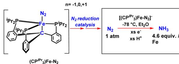
Fig. 30 Ammonia formation using a Fe–N<sub>2</sub> catalyst showing C atom as an anchor.
