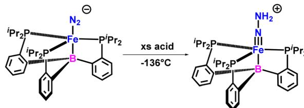
Fig. 31 Fe≡N–NH<sub>2</sub> Intermediate for catalytic Reduction of N<sub>2</sub>.
