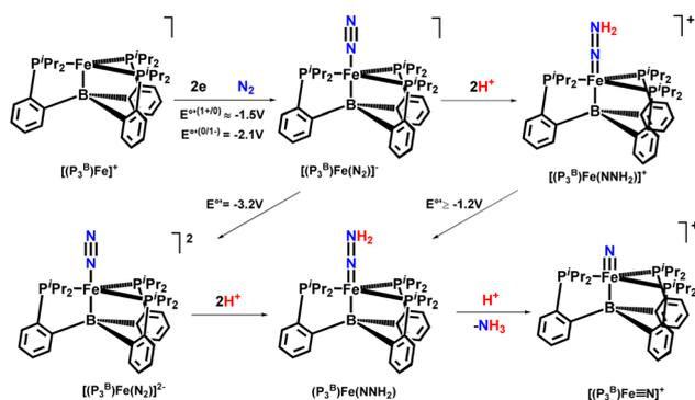
Fig. 36 Nitrogen fixation via a terminal Fe(IV) nitride.
