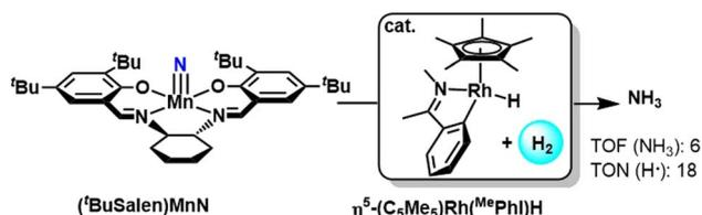
Fig. 42 Hydrogenation of Mn(v) nitride complex for ammonia production.
