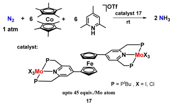
Fig. 20 Ferrocene co-ordinated bis(molybdenum-trihalide) complexes towards ammonia synthesis.
