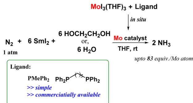
Fig. 23 Ammonia production at ambient reaction conditions by molybdenum complexes formed *in situ* by reacting [Mo<sub>3</sub>(THF)<sub>3</sub>] and monodentate and bidentate phosphines.
