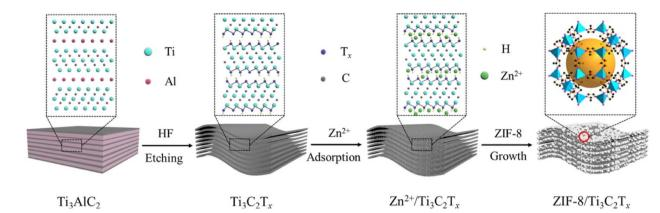
Fig. 3 Illustration of the synthesis of ZIF-8/Ti<sub>3</sub>C<sub>2</sub>T<sub>x</sub>. Reproduced with permission from ref. 86 Copyright ©2022, Elsevier.
