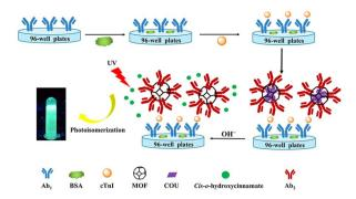
Fig. 4 Schematic diagram of cTnl detection by fluorescence immunosensor with signal amplification. Reproduced from ref. 38 with permission from American Chemical Society.
