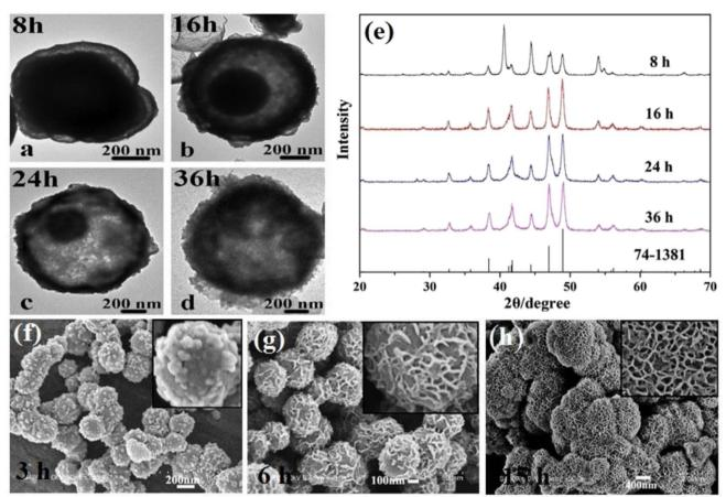
Fig. 3 Effect of synthesis time on: (a) – (d) structure, (e) crystalline phase (reproduced from ref. 60 with permission from Elsevier, Copyright 2015), and (f) – (h) morphology of nickel phosphides. 41
