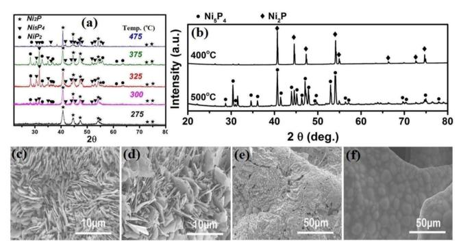
Fig. 6 (a) XRD patterns of nickel phosphides at different temperatures (reproduced from ref. 90 with permission from the American Chemical Society, Copyright 2016) and (b) XRD patterns of nickel phosphides at different temperatures (reproduced from ref. 95 with permission from Wiley, Copyright 2015). SEM images of nickel phosphides at different temperatures of: (c) 400 °C, (d) 500 °C, (e) 600 °C and (f) 800 °C (reproduced from ref. 95 with permission from Wiley, Copyright 2015).
