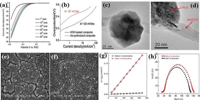
Fig. 9  $N_{13}S_{2}(55\%)/MWCNT-NC$ : (a) LSV curves at different polarization values in 30 wt% KOH and (b) corresponding Tafel plots before and after 12 h base treatment in 30 wt% KOH. (c) TEM image before base treatment and (d) TEM image after base treatment (reproduced from ref. 101 with permission from Elsevier, Copyright 2014). Ni–S/FTO: (e) SEM image before 1 h electrolysis, (f) SEM image after 1 h electrolysis, (g) electrochemical double-layer capacitance and (h) EIS plots.
