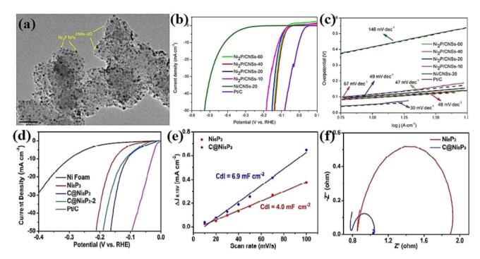
Fig. 14  $Ni_2P$  supported on carbon nanospheres: (a) TEM image, (b) LSV curves in 0.5 M  $H_2SO_4$  and (c) corresponding Tafel plots (reproduced from ref. 78 with permission from Elsevier, Copyright 2015). Carbon-coated  $Ni_8P_3$ : (d) LSV curves in 0.5 M  $H_2SO_4$ , (e) electrochemical double-layer capacitance and (f) EIS plots (reproduced from ref. 108 with permission from the America Chemistry Society, Copyright 2016).
