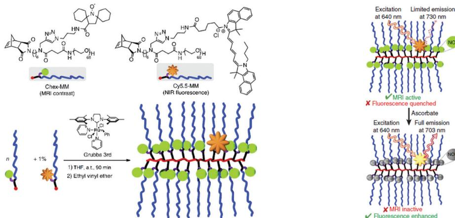
**Scheme 4** Structure of branched bottlebrush polymers bearing nitroxides and fluorophores (left). Concept of MRI and NIR imaging (right). Reproduced with permission from ref. 41. Copyright, Nature Publishing Group, 2014.
