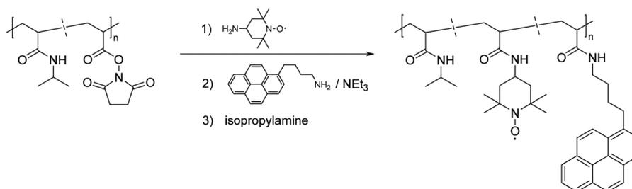
**Scheme 7** Synthetic strategy for implementation of nitroxide based radicals and a pyrene moiety in the PNIPAM backbone.<sup>50</sup>
