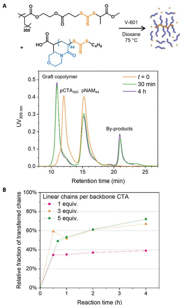
**Fig. 3** (A) SEC data for the transfer of pNAM<sub>44</sub> to pCTA<sub>300</sub> in the presence of V-601 at 75 °C in dioxane.  $A_{UV}$  was normalised for each dataset. Analysis was conducted in DMF with DRI and UV<sub>309 nm</sub> detection and PMMA calibration. (B) Relative fraction of transferred linear chains ( $f_{Rel,UV}$ ), descriptive of the grafting density, plotted against reaction time in reactions with 1 : 1, 3 : 1, and 5 : 1 pNAM to backbone CTA ratios.
