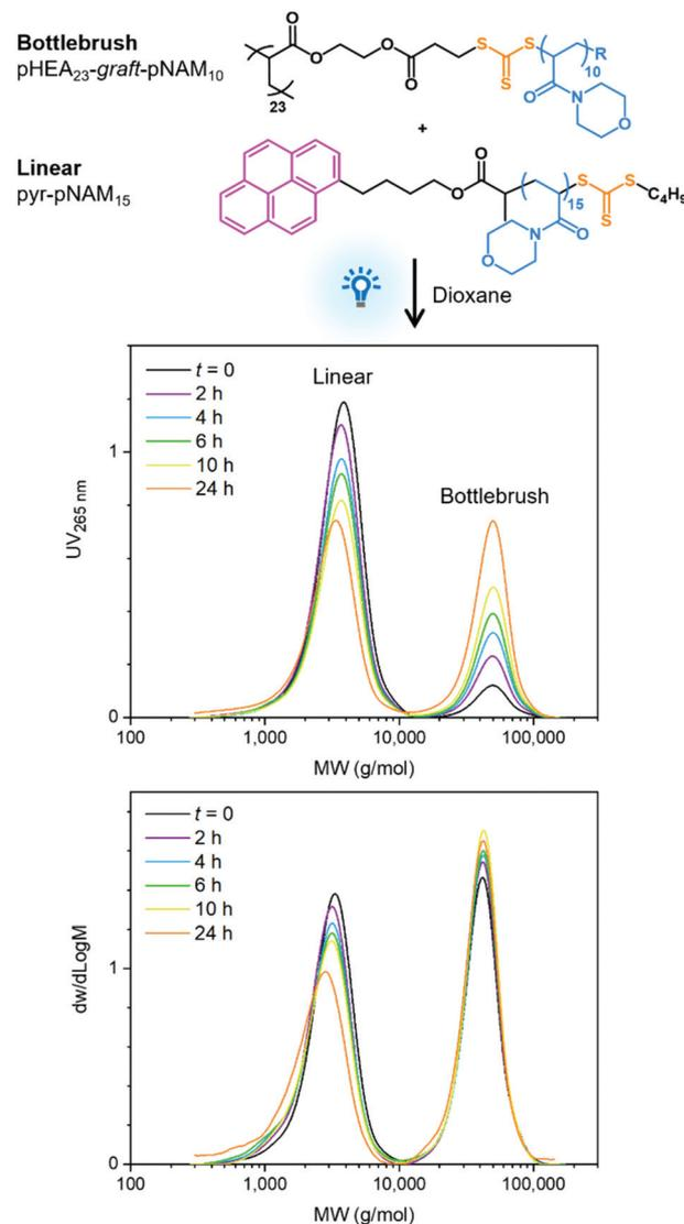
**Fig. 2** SEC data shows exchange of pHEA<sub>23</sub>-graft-pNAM<sub>10</sub> grafts for pyrene-functional linear pNAM<sub>15</sub> chains. Analysis was conducted in CHCl<sub>3</sub> with DRI and UV<sub>265 nm</sub> detection and PMMA calibration.
