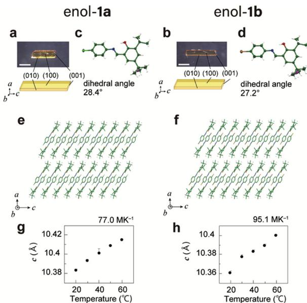
**Fig. 1** Crystal structures of the enol-**1a** and enol-**1b** crystals. (a and b) Photographs and face indices of single plate-like (a) enol-**1a** and (b) enol-**1b** crystals. Scale bars, 1 mm. (c and d) Oak Ridge Thermal Ellipsoid Plot (ORTEP) drawings at 20 °C with a thermal ellipsoid of 25% probability. Disordered *tert*-butyl substituents are indicated in magenta. (e and f) Molecular packing on the (010) side face. (g and h) Temperature dependence of the length of the *c*-axis.
