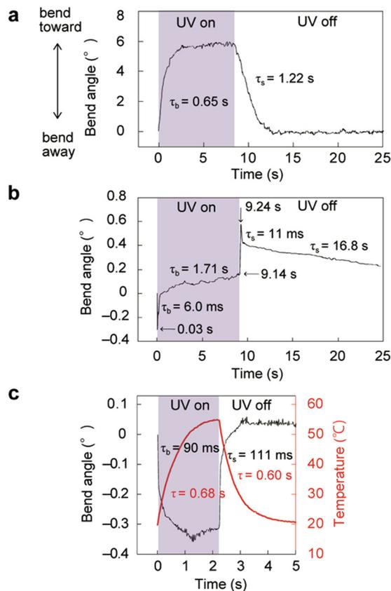
**Fig. 6** Bending of enol-**1b** crystals (Movie S5, ESI†). (a) Thin ( $171 \times 17.2 \times 2.4 \mu\text{m}^3$ ), (b) slightly thick ( $2410 \times 191 \times 65.5 \mu\text{m}^3$ ), and (c) thick ( $2030 \times 344 \times 174 \mu\text{m}^3$ ) crystals bent through photoisomerisation and/or the photothermal effect upon UV laser irradiation of the (100) top face at  $960 \text{ mW cm}^{-2}$  (a and b) and  $230 \text{ mW cm}^{-2}$  (c).
