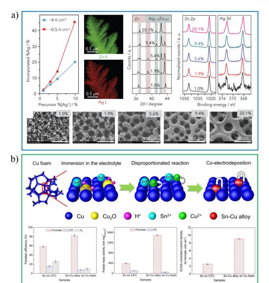
Fig. 4 (a) Ag-Zn alloy growth and characterization. Reproduced with permission.<sup>27</sup> Copyright 2020, Elsevier Inc. (b) Schematic diagram of SnCu alloy preparation and catalytic performance. Reproduced with permission.<sup>28</sup> Copyright 2020, Elsevier.
