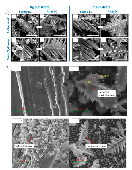
Fig. 3 (a) Scanning electron microscopy (SEM) images of catalysts prepared under different conditions before and after the CDRR reaction. Reproduced with permission.<sup>24</sup> Copyright 2019, American Chemical Society. (b) SEM images of copper and deposits of Bi obtained by different electrodeposition methods: constant potential, CP; direct current, DC; and pulse current, PC. Reproduced with permission.<sup>26</sup> Copyright 2021, Elsevier.
