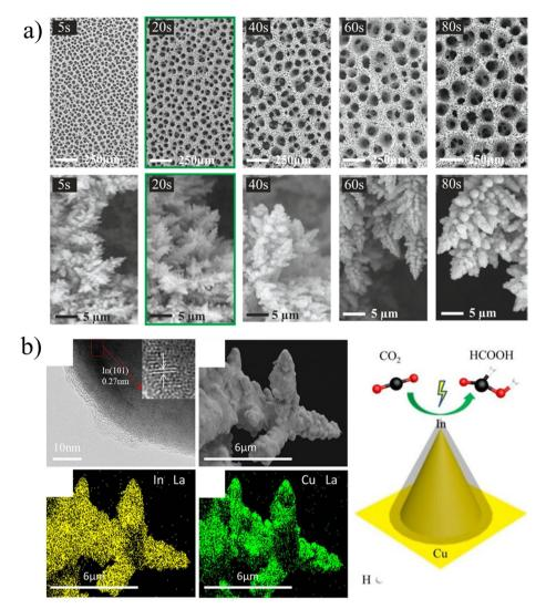
Fig. 7 (a) SEM micrographs showing the changes of surface pore size and dendrite size with deposition time. Reproduced with permission.<sup>46</sup> Copyright 2021, American Chemical Society. (b) HRTEM images of the Cu-In-30 catalyst, SEM image of the Cu-In-30 catalyst, and the corresponding EDX elemental maps. Reproduced with permission.<sup>47</sup> Copyright 2021, American Chemical Society.
