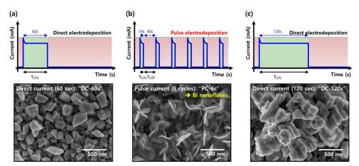
Fig. 5 Current curves and the corresponding SEM images of direct electrodeposition and pulse electrodeposition. Reproduced with permission.<sup>29</sup> Copyright 2017, Elsevier.
