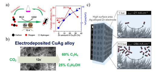
Fig. 10 (a) Schematic diagram of ethanol production from CuZn alloy. Reproduced with permission.<sup>58</sup> Copyright 2016, American Chemical Society, (b) Schematic diagram of the production of C2 products from CuAg alloys. Reproduced with permission.<sup>17</sup> Copyright 2018, American Chemical Society, (c) Schematic diagram of efficient CO production from AgZn alloy. Reproduced with permission.<sup>27</sup> Copyright 2019, Elsevier Inc.
