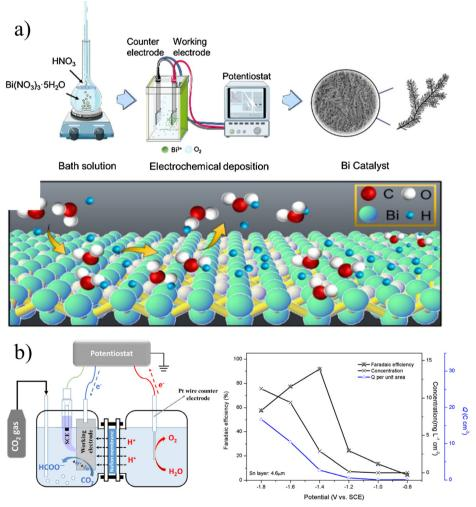
Fig. 2 (a) Schematic diagram of the two-electrode system for constant current deposition of bismuth electrodes. Reproduced with permission.<sup>22</sup> Copyright 2021, Elsevier. (b) Schematic diagram of electrocatalytic reduction of carbon dioxide in a three-electrode system and a summary of its performance. Reproduced with permission.<sup>23</sup> Copyright 2016, Elsevier.
