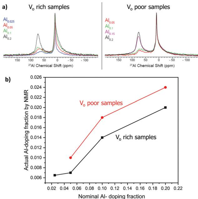
Fig. 6  $^{27}Al$  solid-state NMR. (a) Comparison of 1D spectra; signal intensities are normalized with respect to the sharp signal at ca. 9 ppm. (b) Plot showing the actual and nominal aluminum doping concentration trend for  $V_O$  rich samples made with heating 1 (black curve) and  $V_O$  poor samples made heating 2 (red curve).
