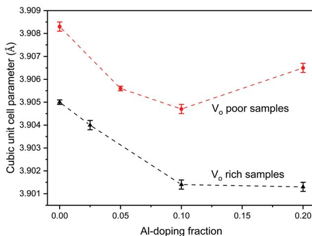
Fig. 4 Change in cubic unit cell parameter of the  $V_O$  rich  $SrTi_{1-x}Al_xO_3$  made with heating profile 1 (black) and  $V_O$  poor  $SrTi_{1-x}Al_xO_3$  made with heating profile 2 (red) as a function of Al doping,  $x$ .
