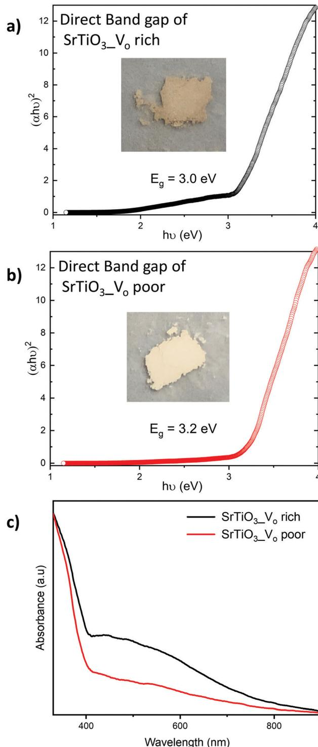
Fig. 7 Tauc plots used to determine direct band gaps of (a)  $V_O$  rich  $SrTiO_3$  obtained via heating profile 1 and (b)  $V_O$  poor  $SrTiO_3$  obtained via heating profile 2. Insets show the images of  $SrTiO_3$  samples obtained via respective heating profiles. (c) UV-Vis spectra of  $V_O$  rich  $SrTiO_3$  obtained via heating profile 1 (black curve) and  $V_O$  poor  $SrTiO_3$  obtained via heating profile 2 (red curve).
