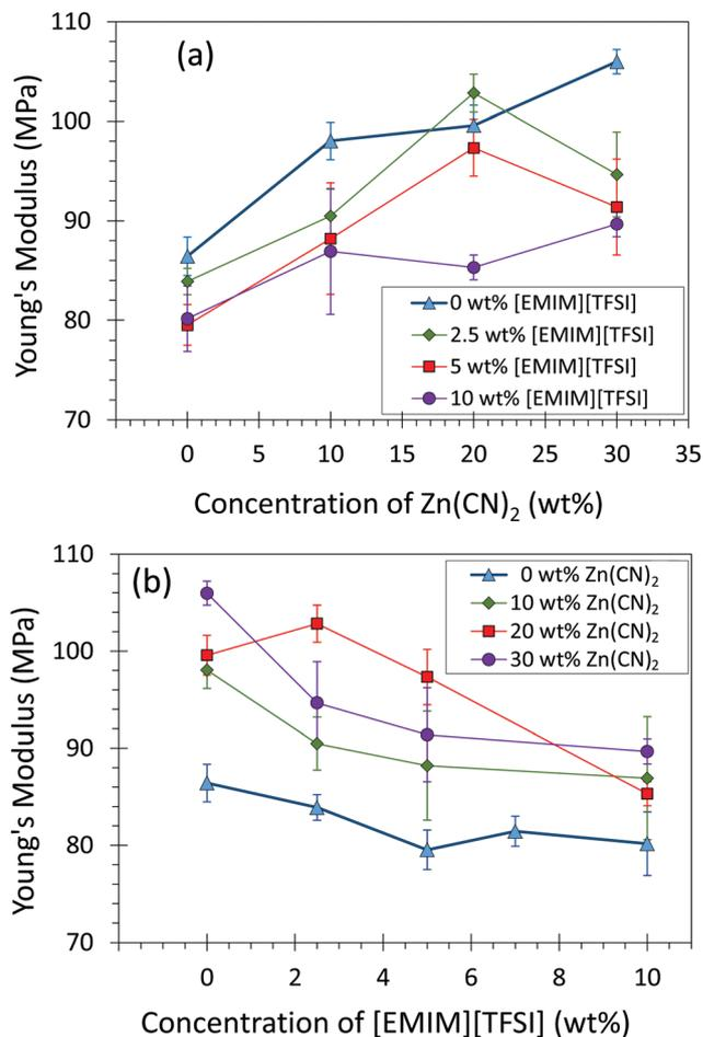
Fig. 3 Young's modulus for LDPE/Zn(CN)<sub>2</sub>/[EMIM][TFSI] composites. (a) Young's modulus slightly increases with the concentration of Zn(CN)<sub>2</sub>, (b) that slightly decreases with [EMIM][TFSI]. Lines are provided to guide the eye. Error bars represent the standard deviation of measurements on replicate samples.
