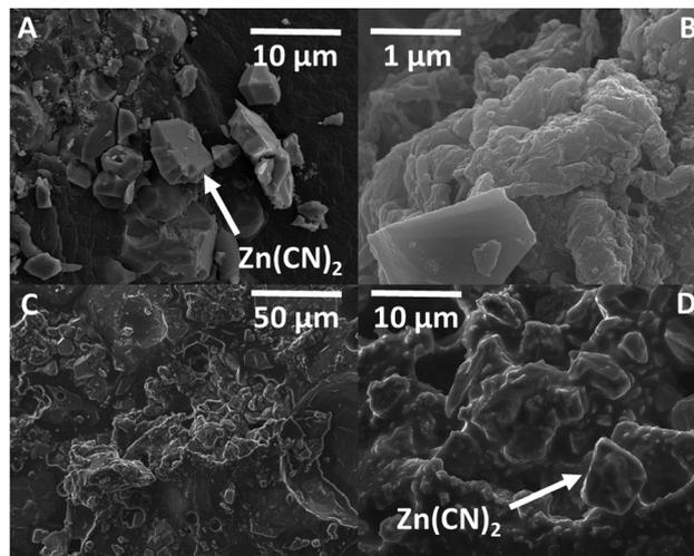
Fig. 1 SEM images of the LDPE/ $\text{Zn}(\text{CN})_2$  interfaces on the fracture surfaces of composites (A) (C-40-0), (B) (C-20-2.5), (C) (C-40-10), and (D) (C-40-10). Note the superior integration of the  $\text{Zn}(\text{CN})_2$  crystallites into the LDPE matrix, indicated by rounded edges, when a sufficient amount of ionic liquid is present.
