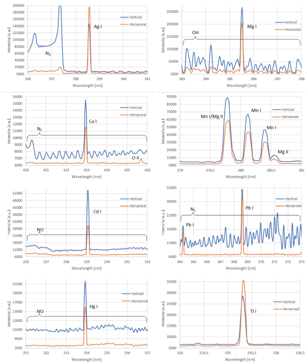
Fig. 6 The morphology of the emission spectra of the HDC-APGD system acquired vertically (along the discharge axis) and horizontally (with the use of the Dove prism) in the vicinity of the analytical lines of Ag, Ca, Cd, Hg, Mg, Mn, Pb and Tl.
