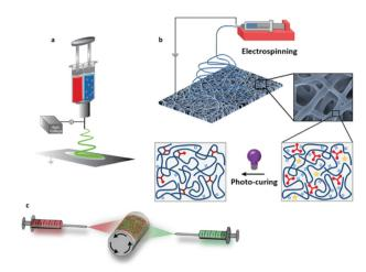
**Fig. 11** Different designs for *in situ* cross-linking strategies: (a) co-axial/double-barrel electrospinning; (b) photo-induced cross-linking; and (c) the development of multi-fiber hydrogel network. (a) Adapted from ref. 199 and (b) adapted from ref. 203 with permission from the American Chemical Society. (c) Adapted from ref. 205 with permission from Wiley-VCH Verlag GmbH & Co. KGaA.
