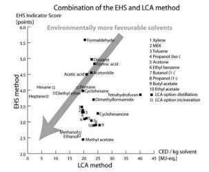
Fig. 1 Classification of 26 solvents by EHS and LCA methods representing the greenest solvents with the lowest scores. Reproduced from ref. 21 with permission from the Royal Society of Chemistry.
