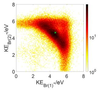
Fig. 9 Correlation diagram between kinetic energies (KEs) of the two Br<sup>+</sup> fragments ions generated in the  ${}^{81}\text{Br}^+ + {}^{81}\text{Br}^+ + \text{CH}^{81}\text{Br}^+$  triple coincidence channel. The result of the CES for synchronous concerted breakup is shown as a green cross "x" symbol.
