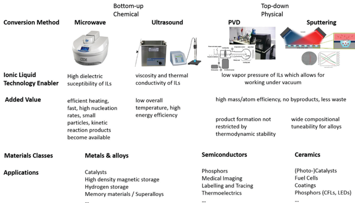
Scheme 1 Bottom-up vs. top-down methods for the synthesis of nanomaterials from ionic liquids.
