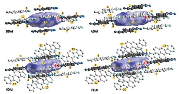
Fig. 4 Hirshfeld surfaces and close contacts in the crystal packing. Black molecules correspond to hydrogen-bonded and  $\pi$ -stacked molecules with respect to the central molecule. Grey molecules complete the close contacts around the Hirshfeld surface. Numbers are included to identify the molecules for the transfer integral calculations.
