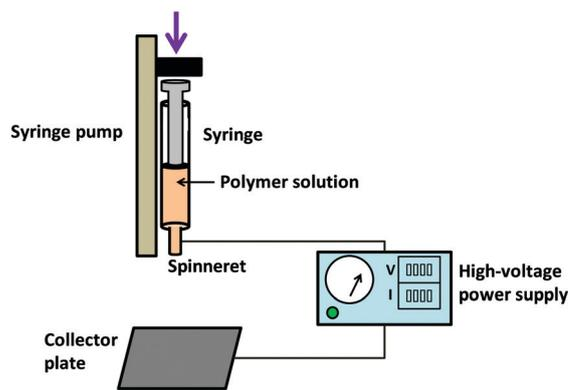
Fig. 2 A schematic illustration of the electrospinning process.
