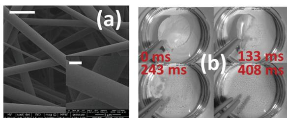
**Fig. 3** (a) Scanning electron microscope images of PVP fibres loaded with paracetamol (21.87% w/w) and caffeine (2.89% w/w) [Scale bars: main image 5 μm; inset 1 μm]; (b) high-speed digital camera images recorded at different after the addition of these fibres to simulated saliva. Adapted with permission from ref. 20 (Illangakoon *et al.*, 2014). Copyright Elsevier 2014.
