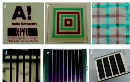
Single-colored  $\text{TiO}_2$  electrodes and modules with dye loading pre-determined by their thickness.
