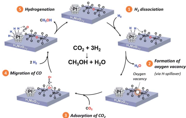
Scheme 2 Proposed reaction mechanism of CO 2 hydrogenation to produce methanol over the Pt/H x MoO 3-y catalyst.
