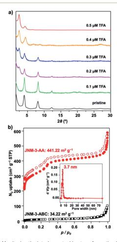
Fig. 2 (a) Monitoring the interlayer stacking transformation by addition of varied concentration of TFA (black, pristine; green to red, 0.1 to 0.5  $\mu M$  TFA). (b) The  $N_2$  adsorption (filled) and desorption (open) isotherm profiles of JNM-3-AA (red cycle) transferred from JNM-3-ABC by addition of 0.5  $\mu M$  TFA and refresh-prepared JNM-3-ABC (black square) at 77 K (inset, the pore-size distribution profiles of JNM-3-AA showing a uniform pore size of  $\sim\!3.7$  nm.).
