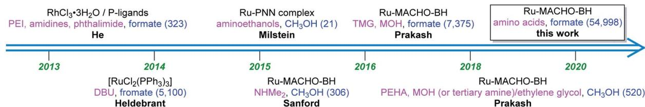
Fig. 1 Representative catalysts and absorbents for CO<sub>2</sub> hydrogenation to C1 products applied in CCU processes. The highest TON (turnover number) of formates or methanol are shown in parentheses, respectively.
