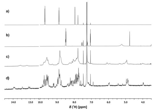
Fig. 7 Partial <sup>1</sup>H NMR (500 MHz, CDCl<sub>3</sub>) spectra of (a) c-P6 (0.16 mM, 298 K), (b) a 1:1 mixture of pB3 and mA2 (0.48 mM, 298 K), (c) a 1:3:3 mixture of c-P6 (0.16 mM), pB3 and mA2 (0.48 mM) at 298 K, and (d) a 1:3:3 mixture of c-P6 (0.16 mM), pB3 and mA2 (0.48 mM) at 233 K.
