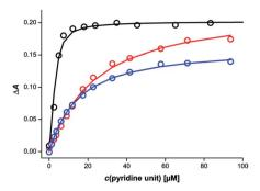
Fig. 6 UV-vis-NIR titration data (CHCl $_3$ , 298 K) for addition of mB3 (red), mA1 (blue) or a 1:1 mixture of mB3 and mA1 (black) to c-P6 (0.7  $\mu$ M). The absorption at 838 nm is shown as circles, and the lines are the calculated best fit to a 1:1 binding isotherm assuming that the six porphyrin units of c-P6 act identically and independently.
