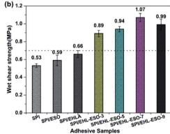
Fig. 7 Wet shear strength of plywood bonded by different soy protein-based adhesives: (a) the schematic diagram of test instrument, (b) the results of wet shear strength.
