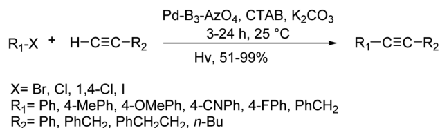
Scheme 61 The Sonogashira reaction in the presence of the Pd-B 3 -AzO 4 .
