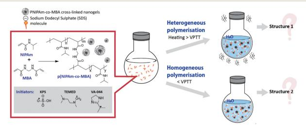
Fig. 1 Scheme of synthesis of pNIPAm-based crosslinked gels by heterogeneous and homogeneous polymerisation.
