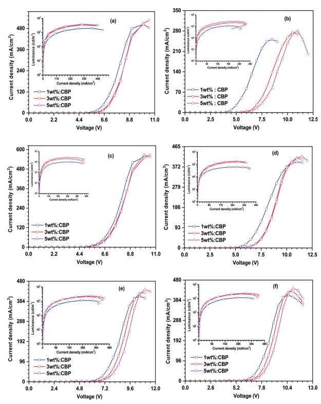
Fig. 7 Current density-voltage-luminance relationship of the dyes (a) 27PI36CN, (b) 27CN3PI, (c) 27PHPI, (e) 27PHPI3CN and (f) 27PHPI36CN.
