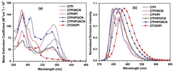
(a) Absorption and (b) emission spectra of the dyes recorded in dichloromethane solution
