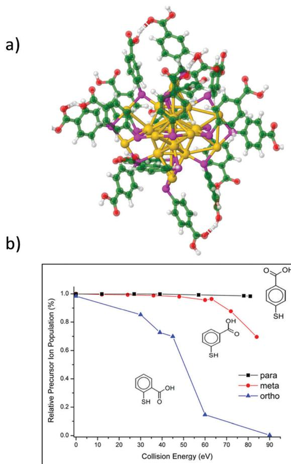
Fig. 10 (a) Proposed structure for Au<sub>25</sub>(MBA)<sub>18</sub> with *p*-MBA isomeric ligand. (b) CID breakdown curves for the 4-charge state of Au<sub>25</sub>(MBA)<sub>18</sub> for the three isomeric MBA ligands as a function of collision energy. (reprinted with permission Copyright © 2018 American Chemistry Society).<sup>216</sup>
