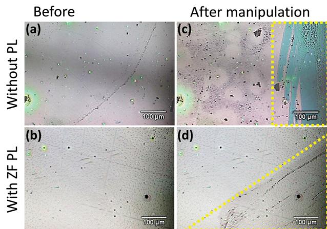
Fig. 4 Optical microscopy photographs of the surface of Tamm plasmon devices with and without PL.  $4\times(\text{SB}/\text{TF})/\text{Au}$  and  $4\times(\text{SB}/\text{TF})/\text{Au}/\text{ZF}$  before (a and b) and after (c and d) macroscopic damage due to manipulation. The yellow dotted lines in (c and d) mark the areas that underwent simulated mechanical manipulation.
