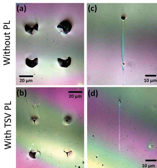
Fig. 5 Optical microscopy photographs of the surface of Tamm plasmon devices with and without PL. Array of 4 indentations up to 1000 nm depth in  $4\times(\text{SC}/\text{TB})/\text{Au}$  (a) and  $4\times(\text{SC}/\text{TB})/\text{Au}/\text{TSV}$  (b); scratches in the same Tamm plasmon devices, without (c) and with (d) TSV PL.
