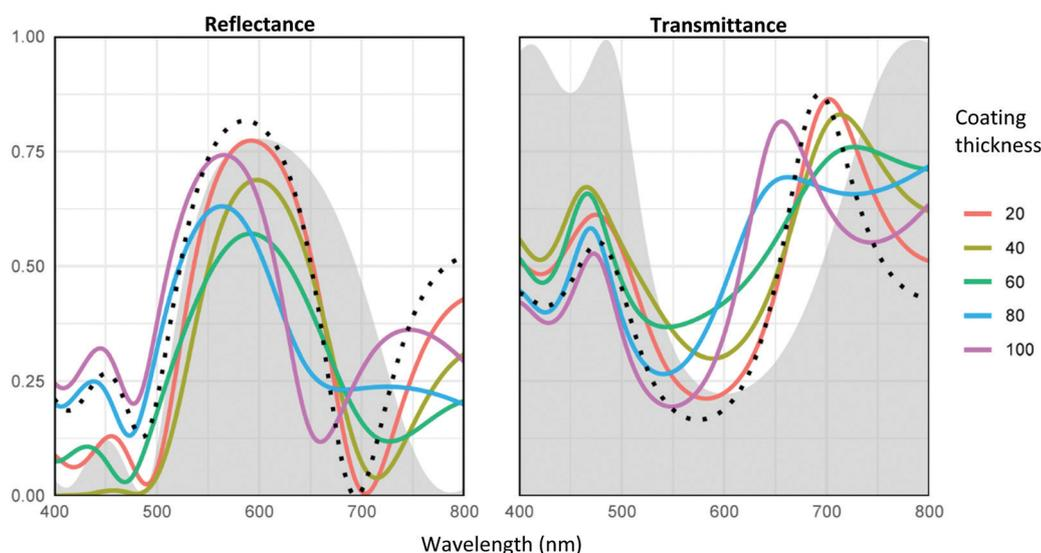
**Fig. 1** Variation of the reflectance (left) and the transmittance (right) spectra of a Tamm plasmon device with the incorporation of a superficial PL of different thicknesses from 20 to 100 nm. The grey shadows represent the corresponding DBR spectra (*i.e.* the device without the Au layer). The dotted black line corresponds to the bare TPP structure (no PL layer).
